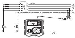
For this example max value is  $1667\Omega$ , the loop tester reads  $12.74\Omega$ , it means that the condition **RA**  $\leq$  **50/la** is respected.
