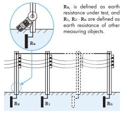
Of these earth resistances,  $R_1$ ,  $R_2$ ,  $\cdots$   $R_n$ can be considered that they are connected in parallel.
