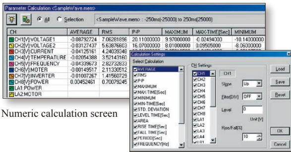
19 types of numerical calculations can be displayed for all the areas or a specific area only. In addition to effective value, maximum value, frequency, and other standard values, you can also calculate values for characteristics such as duty ratio and rise time.
